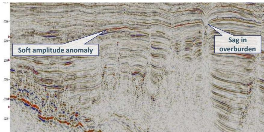
Seismic example showing soft amplitude anomaly with apparent fluid pipe termination at the anomaly. Line also shows a sag feature above fluid pipe.
