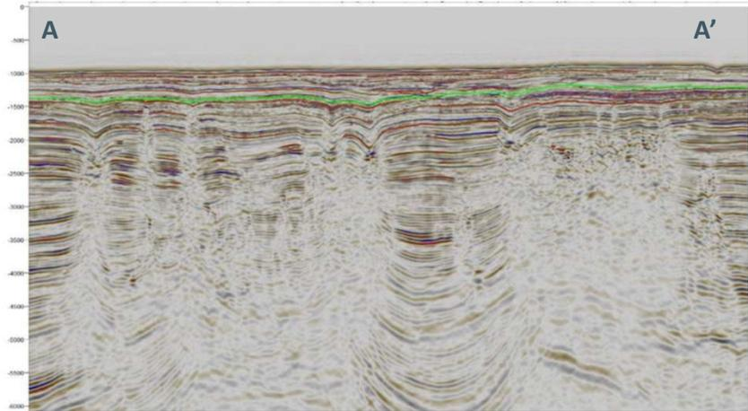
Arbitrary seismic amplitude (above) & variance (below) sections from eastern part of 3D indicating fluid escape features terminating at Mid Miocene level
